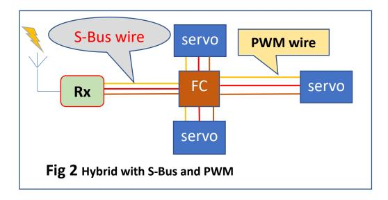
So, they switch the yellow wire on and off in a predetermined sequence 25 times within a 10 millionth of a second (0,1,1,0,0,1,1....) then stop. That is the instructions set for a given channel, say the rudder; they call it a packet. The next set of 25 'pulses', or packet, might be for the ailerons, then stop. The packet looks something like fig 4. Fig 5 is a close-up showing the 'on' or 'off' with the on or off sometimes repeated looking like a bar.
