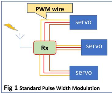
Skipping the standard '*pulse width modulation system*' (PWM) which we balsa wood flyers use as in Fig 1; we need to understand bus systems.
