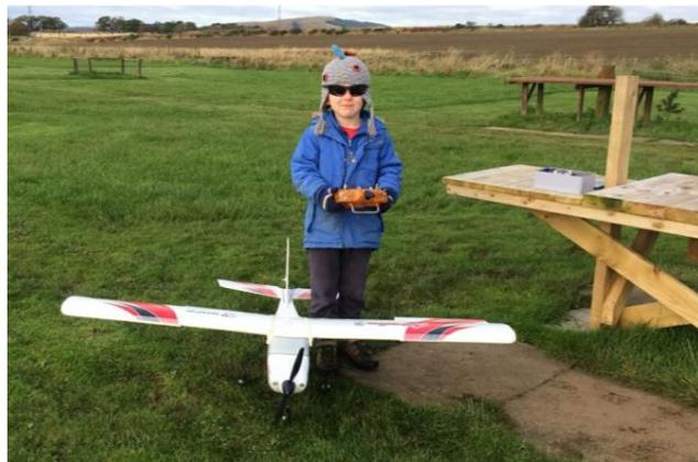
My kingfisher high wing plane is fitted with a wind gyro. This allows the plane to fly in full control but will counteract any outside influences such as the wind pushing the plane in any direction. It simply allows me to fly in higher wind speeds than normal. It does not limit any of the controls on the plane, but just makes flying it like you're flying in calm skies. The rate of input from the gyro is fully adjustable from the transmitter by a slider switch, or can be switched off completely.
