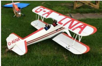
More controversially, my Stearman biplane is fitted with a helicopter tail gyro which simply means that it won't ground loop on take-off. This gyro, however, if it was left switched on in the air would mean that the plane would not turn at all, so a means to switch it off once the plane has taken off is essential. It hasn't happened yet but if this was to go faulty it would result in the plane being un-flyable. People
